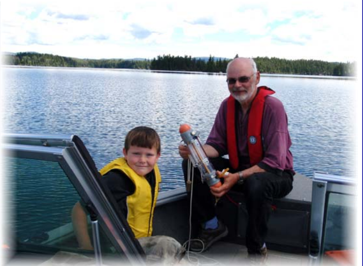
Above left: Justin Swan holds the collector jar with the 50 micron screen, retaining all the zooplankton collected in the net. Above right: Justin Swan and Karl Schmitz draw the student point sampler up from the lake, which contains a water from a specific depth.
