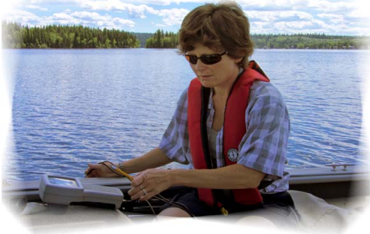
Chris Swan checks the water temperature and oxygen levels at 2 meter intervals from the lake surface down to the lake bottom in over 30 meter depth.
